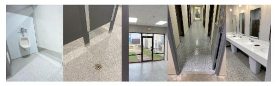
An optimal solution for addressing challenges in high-traffic restrooms, kitchens, and dining areas. This flooring features approximately 1/4" of urethane-modified cement underlayment, topped with your selection of vinyl chip blend aggregates, all encapsulated and sealed with chemically-resistant epoxies and urethanes.
